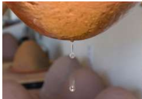
Figure 3. A ceramic water filter jointly developed by ceramic scientists, artists and engineers provides potable water in isolated communities (Credit: B. Stephen Carpenter II).
