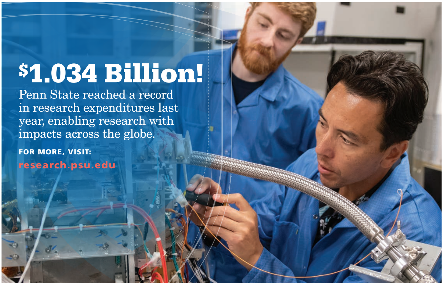
Randall McEntaffer, head of Penn State's Department of Astronomy and Astrophysics, makes adjustments to the flight electronics and power supply of the X-ray spectrometer that he and his team built for a September launch with NASA. Credit: Patrick Mansell / Penn State. Creative Commons.
